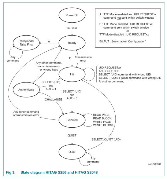
**Remark:** Switching off the powering magnetic field or moving the HITAG S Transponder out of the RWD antenna field enters the HITAG S Transponder into the Power off state independently of its actual state.
