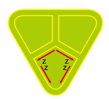
7 | INSTALL THE NEW CANOPY, Find the zipper head and install the canopy in the direction of the arrow
