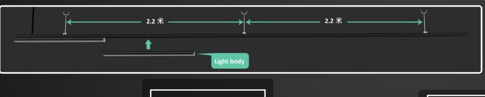
C: Clip the lamp body upwards into the bridge
