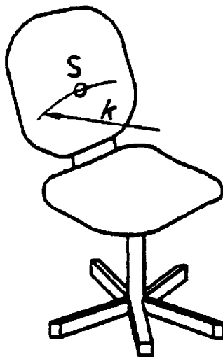
Figure 13 - Determination of the horizontal radius k of the back rest
