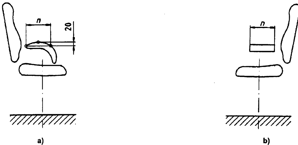
Figures 15 - Determination of the length n of the useful area of the arm rest
