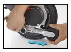
6. As shown in Fig. F6, press the anti-tipping wheel button and pull out the anti-tipping wheel.
