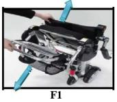
1. As shown in Fig. F1, pull out the chair by holding the position shown in the figure as directed by the arrows.
