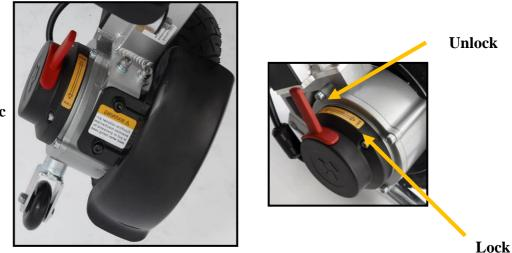
Electromagnetic Brake Lever
