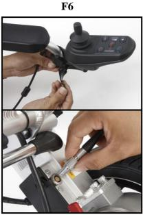
7. Mount the control panel and plug in the 4 –pin control cable in accordance with Fig. F7. (refer to the instructions on mounting the Control Panel)
