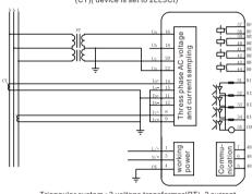
Triangular system: 2 voltage transformer(PT), 2 current transformers(CT)( device is set to 2LL2Ct)
