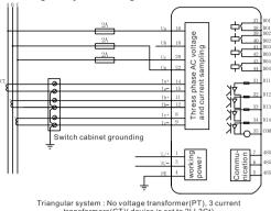
Triangular system : No voltage transformer(PT), 3 current transformers(CT)( device is set to 2LL3Ct)
