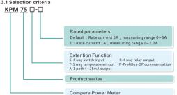
Example:KPM75T-1:Rate current 380V/1A,1 way temperature input, Power quality analysis meter.
