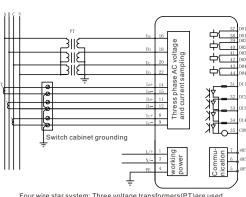
Four wire star system: Three voltage transformers(PT)are used. (The device is set to 3Ln3Ct)
