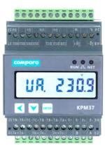
KPM37 Three Phase Rail Smart Power Meter adopts DIN 35MM rail type installation structure and LCD display. It integrates three-phase electric parameter measurement, 2~31st harmonic analysis and time statistics.KPM37 default communication is Modbus-RTU by RS485 interface. WiFi, 4G, Lora communication are optional. The meter can also expand 2-way digital input and 2-way relay output, 4-way temperature measurement and 1 way residual
