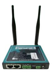
The KPM201 communication gateway completes the information interaction between the microcomputer protection, automatic device, measurement and control of the power distribution room and the computer system and the power grid automation system.
