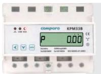
KPM33 three-phase smart energy meter with DIN35mm type installation structure, LCD display, measurement of electrical energy and other electrical parameters, it can set some parameter, such as the clock, rate period, and so on, it also own electrical energy pulse output function; default RS485 communication interface, optional WIFI connection.
