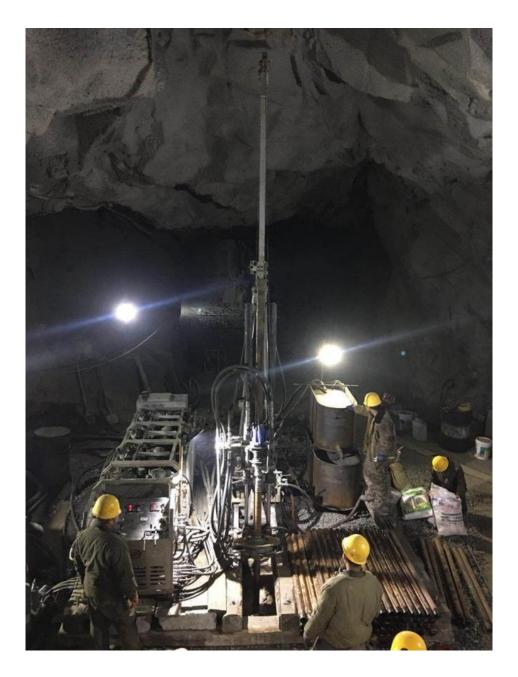
One exploration company in north China used our HTW/NTW drill rods, HTW/NTW core barrels, NTW/HTW diamond bit in one of their drilling projects in gold prospecting.
