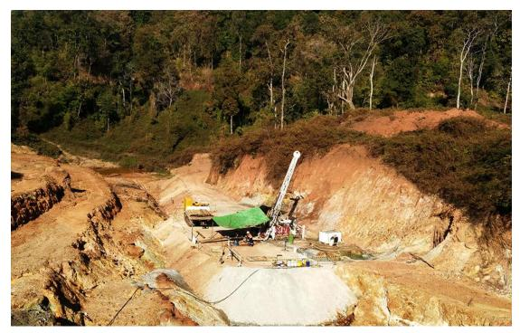
One exploration company in Myanmar used our PHD/HQ/NQ drill rods, PQ/HQ/NQ core barrels, PQ/HQ/NQ diamond bit in one of their drilling projects in copper prospecting.
