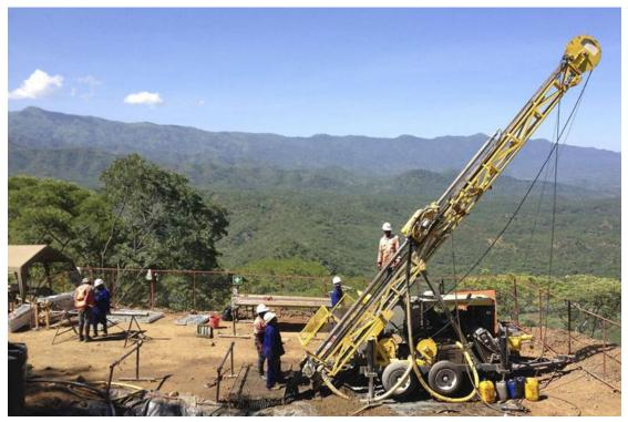
One exploration company in Tanzania used our HWT casing, HQ/NQ drill rods, PQ/HQ/NQ core barrels, PQ/HQ/NQ diamond bit in one of their drilling projects in gold prospecting.
