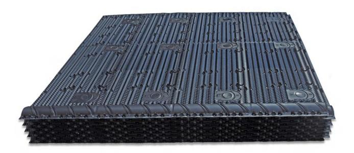
Newin BAH Film Fill is a hanging film type cooling tower fill which incorporates highly efficient cellular drift eliminator and molded with the air inlet louver, spreads the water through the thin film, flowing over large vertical surfaces, promoting maximum exposure to air flow to get higher cooling efficiency. This type of fill provides much more water surface exposure per cubic foot than splash type fill.
