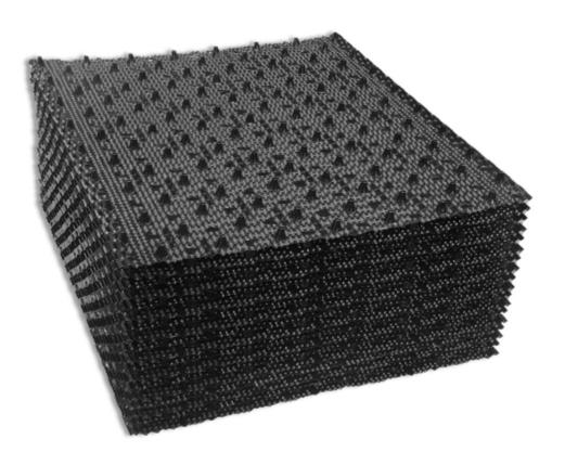
Newin LAH Film Fill is a hanging film type cooling tower fill which incorporates highly efficient cellular drift eliminator and molded with the air inlet louver, spreads the water through the thin film, flowing over large vertical surfaces, promoting maximum exposure to air flow to get higher cooling efficiency. This type of fill provides much more water surface exposure per cubic foot than splash type fill.
