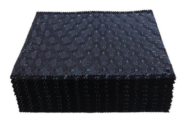
Newin SPH Film Fill is a hanging film type cooling tower fill which incorporates highly efficient cellular drift eliminator and molded with the air inlet louver, spreads the water through the thin film, flowing over large vertical surfaces, promoting maximum exposure to air flow to get higher cooling efficiency. This type of fill provides much more water surface exposure per cubic foot than splash type fill.
