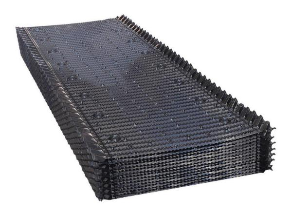
Newin HOH Film Fill is a hanging film type cooling tower fill which incorporates highly efficient cellular drift eliminator and molded with the air inlet louver, spreads the water through the thin film, flowing over large vertical surfaces, promoting maximum exposure to air flow to get higher cooling efficiency. This type of fill provides much more water surface exposure per cubic foot than splash type fill.
