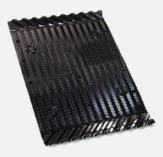
A hanging design type cooling tower fill spreads the water into a thin film, flowing over large vertical surfaces, promoting maximum exposure to air flow.
