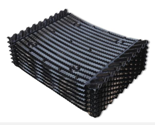
Newin MEH Film Fill is a hanging film type cooling tower fill which incorporates highly efficient cellular drift eliminator and molded with the air inlet louver, spreads the water through the thin film, flowing over large vertical surfaces, promoting maximum exposure to air flow to get higher cooling efficiency. This type of fill provides much more water surface exposure per cubic foot than splash type fill.
