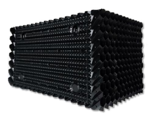
Newin RYH Film Fill is a hanging film type cooling tower fill which incorporates highly efficient cellular drift eliminator and molded with the air inlet louver, spreads the water through the thin film, flowing over large vertical surfaces, promoting maximum exposure to air flow to get higher cooling efficiency. This type of fill provides much more water surface exposure per cubic foot than splash type fill.
