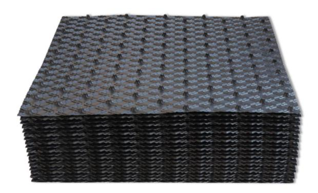
Newin TCH Film Fill is a hanging film type cooling tower fill, spreads the water through the thin film, flowing over large vertical surfaces, promoting maximum exposure to air flow to get higher cooling efficiency.
