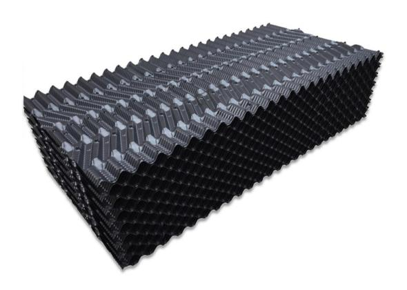
Newin HAN Film Fill Applicable for Hamon cooling tower, any induced draft or natural draft cooling tower, specially designed to induce highly turbulent mixing of the air and water for superior heat transfer. The fill is constructed of PVC, the structural integrity of the fills is greatly enhanced, excellent fire resistant qualities.
