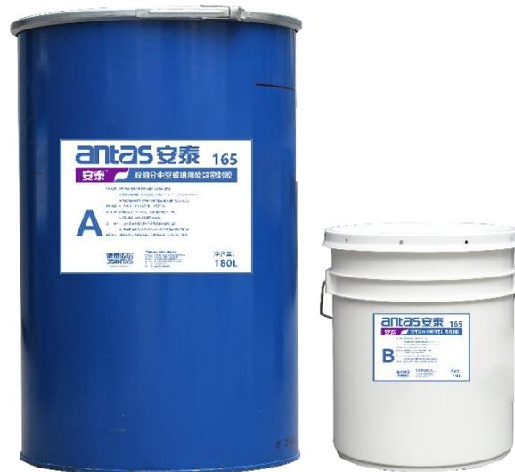
antas-165 is two-component, non-structural, neutral-curing insulating glass sealant. It is used as the secondary sealing in an insulating glass unit. It has good adhesion to most building materials without corrosion or stain to metal, glass, concrete, marble and etc. It has excellent weathering performance with over 15 years' service life under general environment. The service temperature is  $-50^{\circ}\text{C} \sim 150^{\circ}\text{C}$ .
